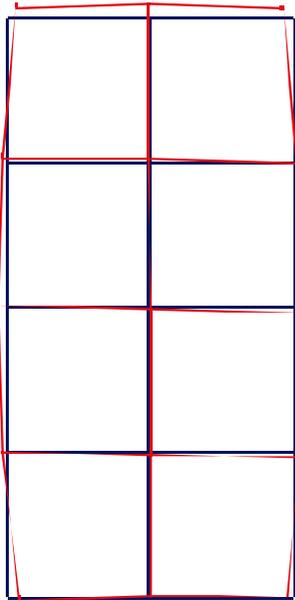
Figure 1. Effect of adjusted self-calibration parameters (in red) scaled by a factor of 1000
