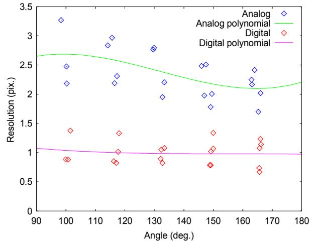
Figure 5. Measurements of resolution and fitted polynomials for analog (blue and green) and digital images (red and pink) against angle in image.
