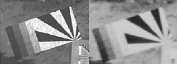
Figure 3. Digital (left) and analog (right) images of the 11-sector resolution target
